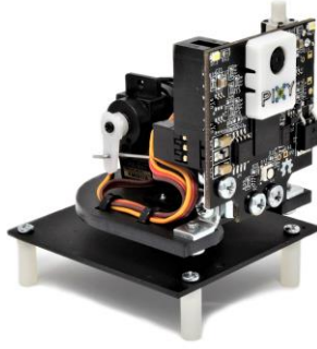
Figure 2. Pixy2 CMUcam5 vision-sensor camera used in this work
