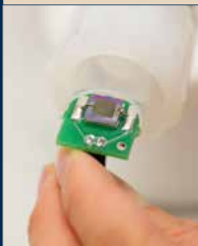
This close-up image shows a functionalized nanomaterial-based chemical sensor, inside a flow-cell test chamber.
