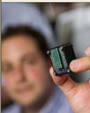
Milad Navaei, a graduate research assistant, holds the micro gas chromatograph, which is being developed by GTRI researchers for early detection of diseases in crops.
