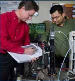
Professor John Cressler (left) and graduate student Partha Chakraborty work at a cryogenic probe station at Georgia Tech to analyze the operation of the new silicon-germanium chip.
