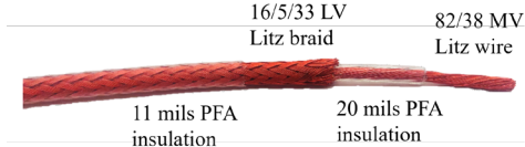
Fig. 9. Coaxial Litz cable for the MFT prototype to achieve low leakage and high insulation voltage at the same time.
