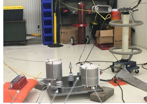
Fig. 15. Lightning-protection-component test setup. A 90 kV 1.2 \mu s/50 \mu s impulse generator is connected to the setup.
