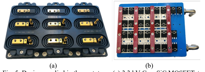
Fig. 5. Devices applied in the prototype. (a) 3.3 kV Cree SiC MOSFET + SiC diode reverse-blocking module. (b) 650 V self-assembled Si IGBT + SiC diode module on a heatsink.
