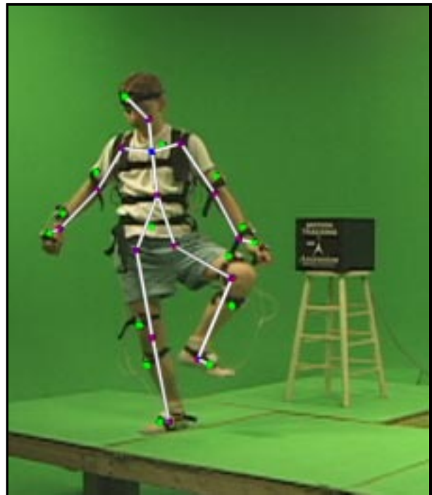
Figure 1: Test subject and generated model. The image shows a subject wearing the motion capture equipment during a capture session with the skeletal model generated automatically from the acquired motion capture data superimposed. The chest and pelvis sensors are on the subject's back.
