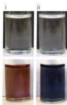
Figure 2.1.1 Titanium Oxide Hydrate Photochromism. The photochromic response of titanium oxide hydrate/glycerol hybrids is visible by eye and depends on the species of titanium oxide hydrate, mononuclear (i) or polynuclear (ii), and unirradiated (top) or irradiated (bottom) (6).
