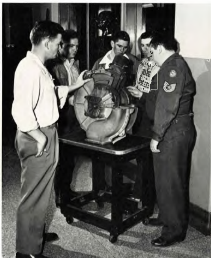
Cut-away turbo supercharger.
