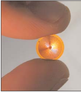
The CardioMEMS sensor is based on technology originally developed at the Georgia Institute of Technology for monitoring jet engines.
