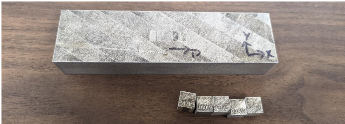
Figure 92: Cross cut of additional 316L PBF specimen
