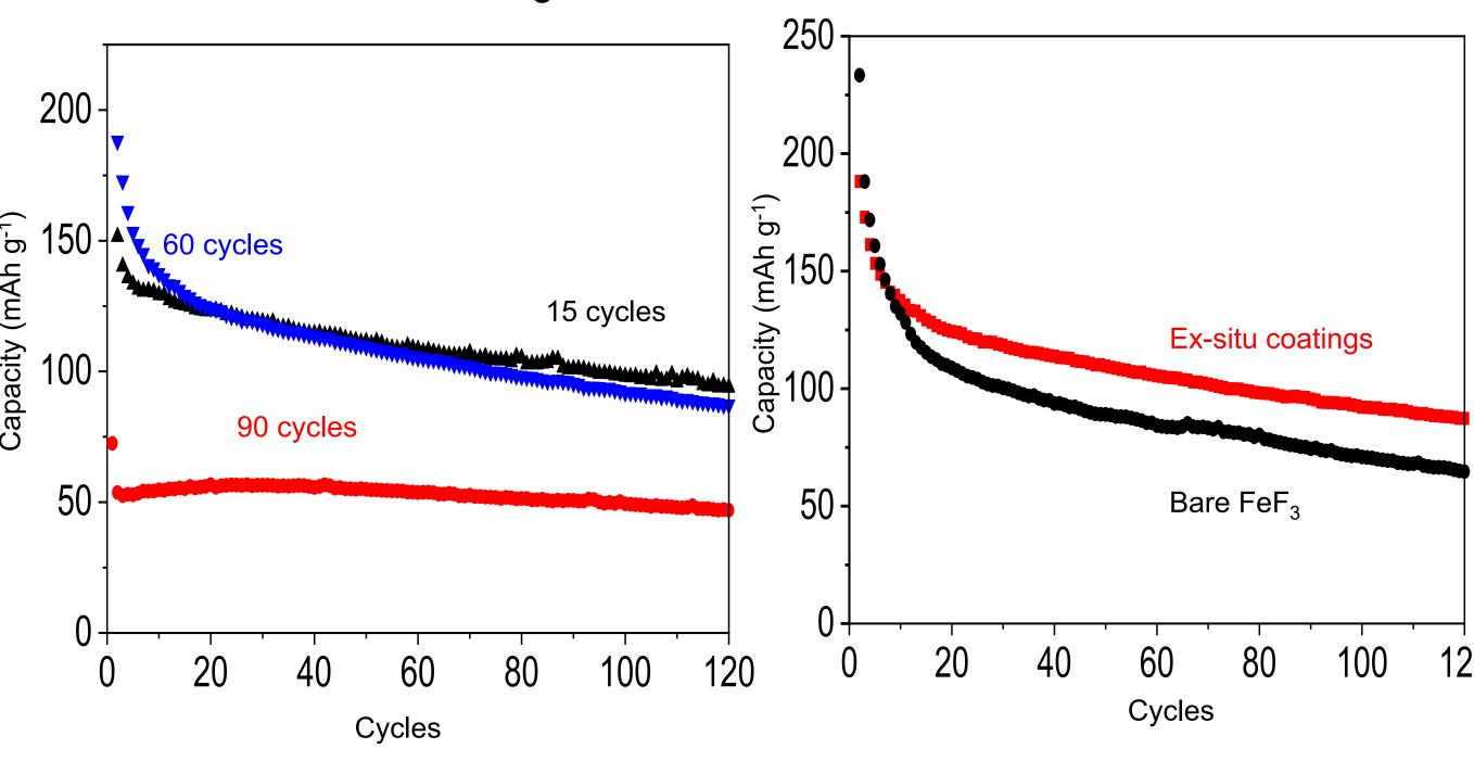
Ex-situ formed coatings improved the cycling stability of FeF<sub>3</sub> in the first 120 cycles and 15 ALD Al<sub>2</sub>O<sub>3</sub> coatings performed the best when comparing coatings with other ALD cycles.
