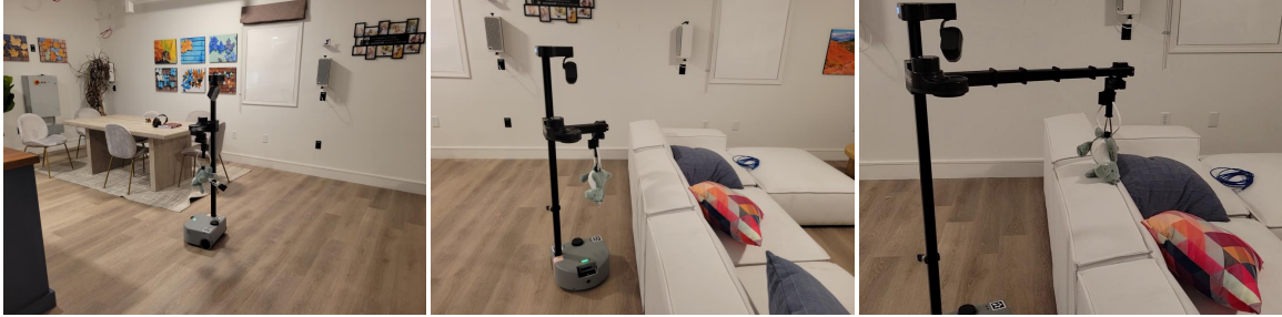
Figure 3.3: An example of the robot navigating to a goal receptacle (sofa) and using the heuristic place policy to put down the object (stuffed animal). Heuristic policies provide an interpretable and easily extended baseline.
