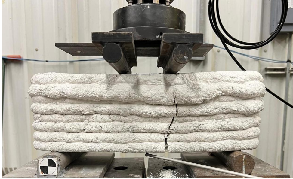
Fig. 3.2. Flexural testing of printed beam specimens.
