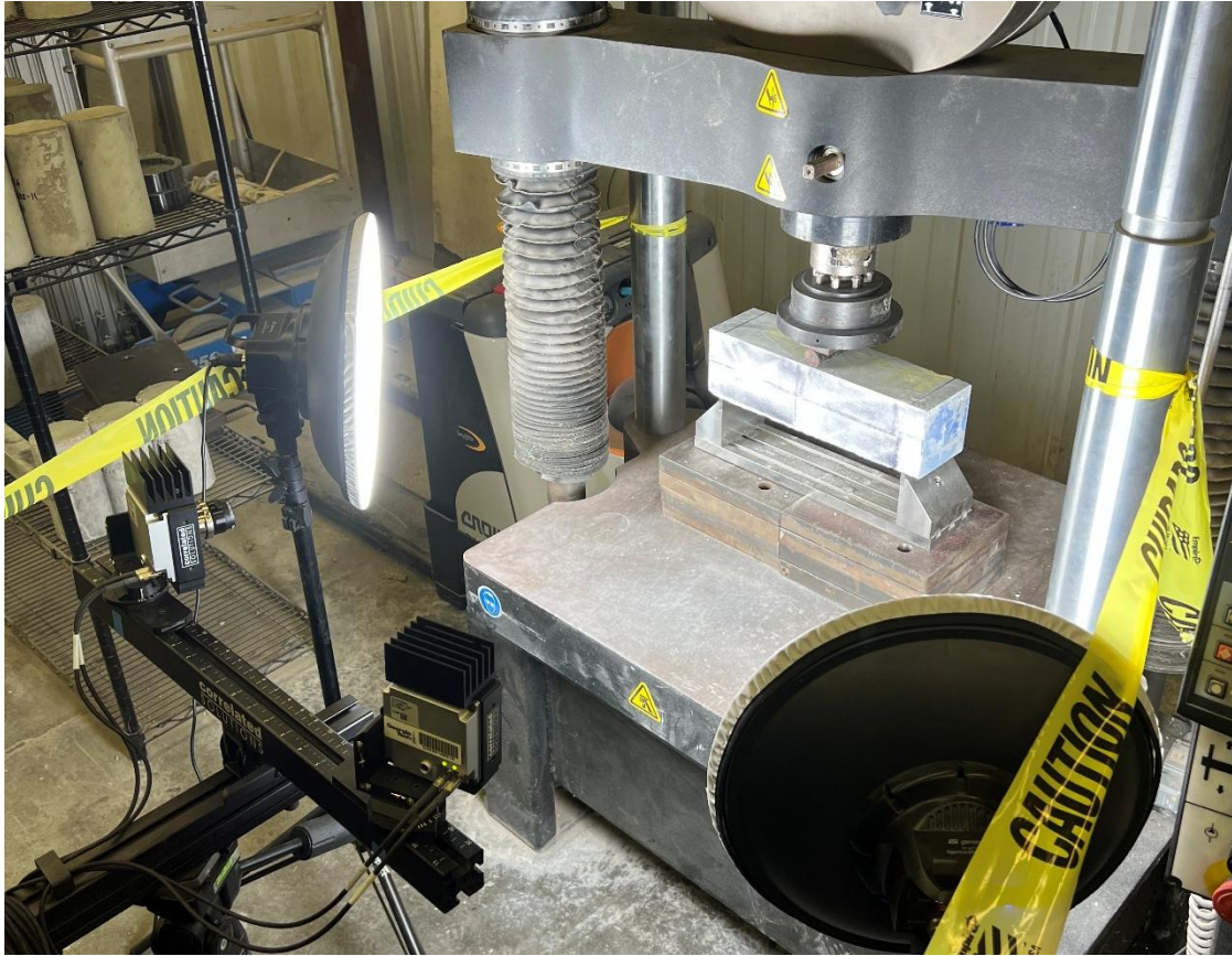
Fig. 5.5. Testing setup for digital image correlation.
