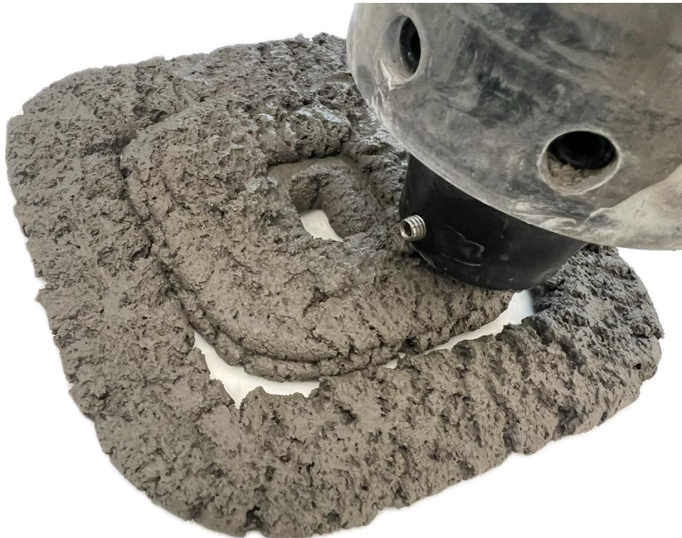
Fig. 4.11. Printing of the mortar designed from candidate mixture I.
