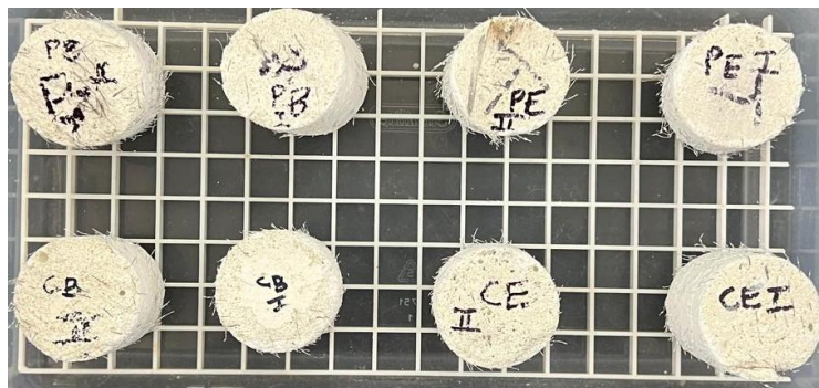
Fig. 3.3. Sorptivity testing of cores from printed and cast beam specimens.
