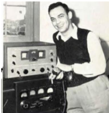
Figure 4-5 - Club president James Elliott shows off some of the equipment in the shack in 1954. The receiver on top is a Hammarlund HQ-129X. Below the receiver is the BC-610 transmitter (Blueprint, 1954).
