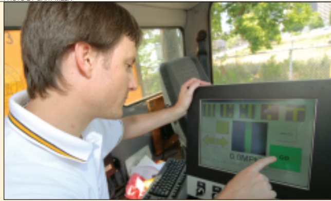
ABOVE: GTRI researcher Colin Usher uses a touch-screen monitor mounted in the cab of the truck. It provides the primary operator interface to the automated raised pavement marker (RPM) placement system developed by GTRI.
