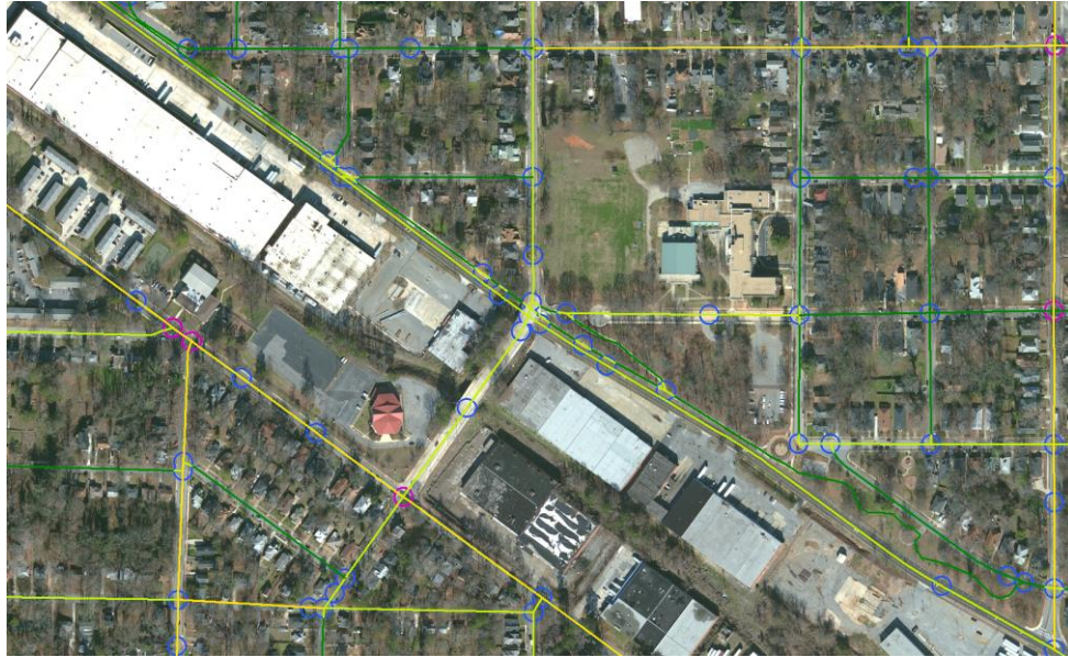
Figure 14: Close up section of the LTS network and the signalized (purple) and unsignalized (blue) intersections.
