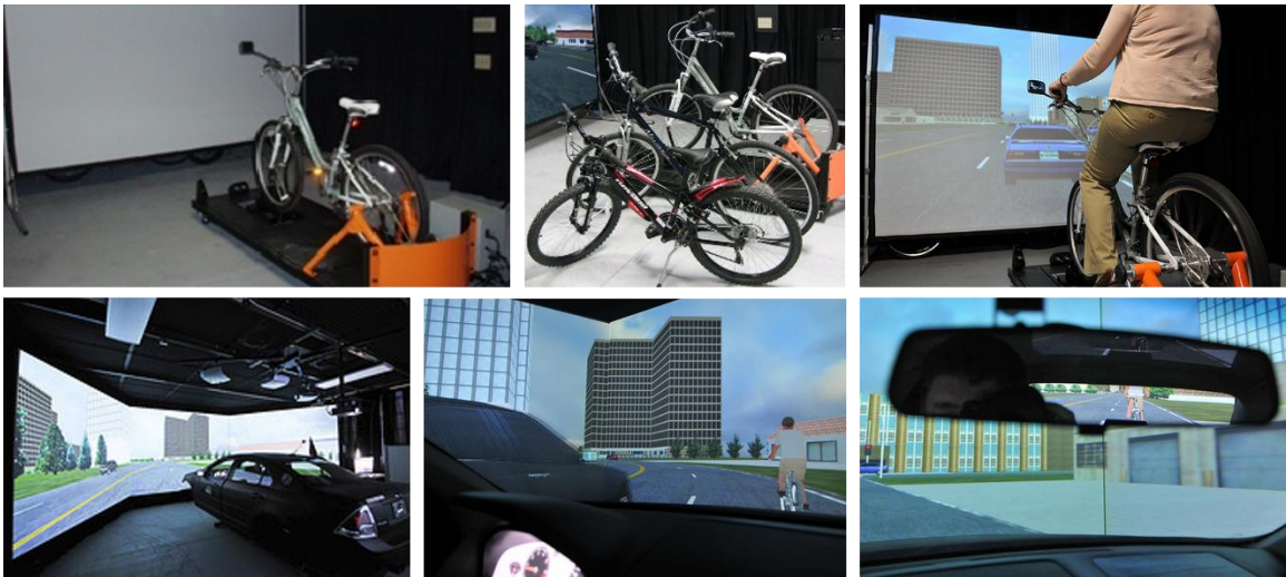
Figure 31: Oregon State University Bicycle Simulator interacts with Vehicle Simulation (Hurwitz Research Program, 2015; Jonathan Maus, 2011)
