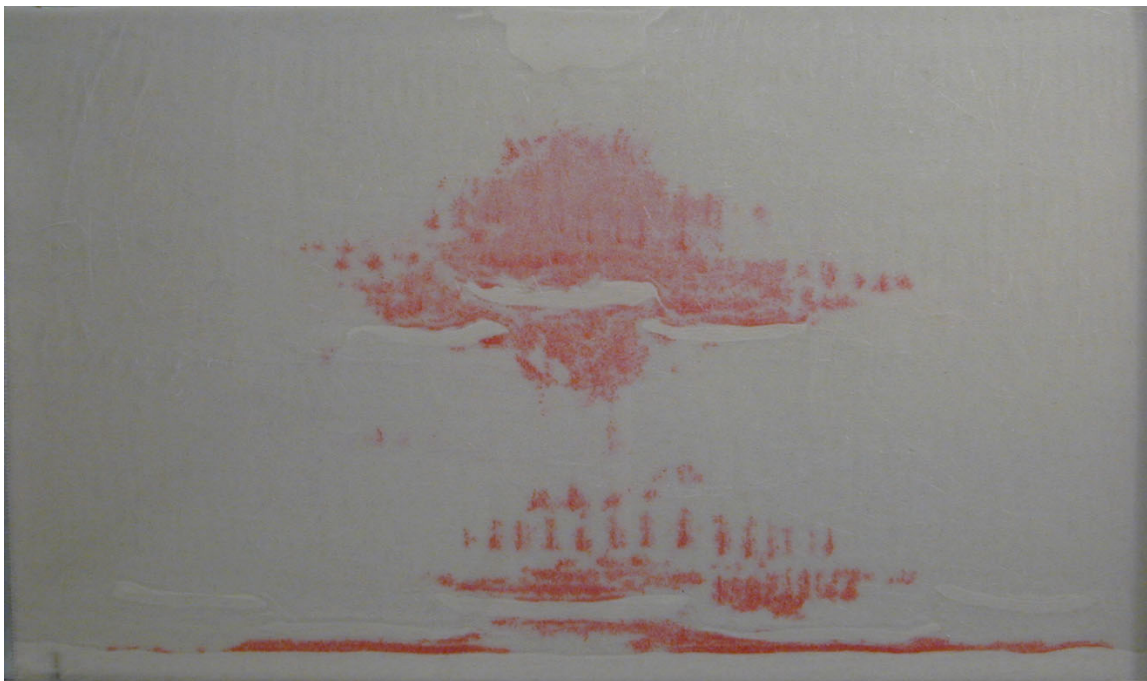
Figure 6.2: Photograph of initial PCE-DNAPL saturation distribution in DMD-HI aquifer cell.
