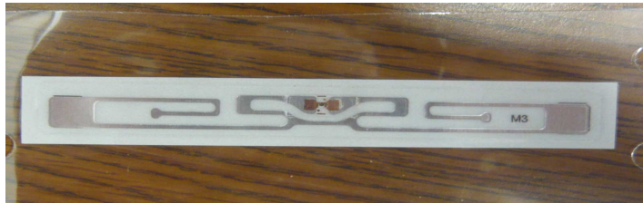
Figure 2.2: Passive RFID tag
