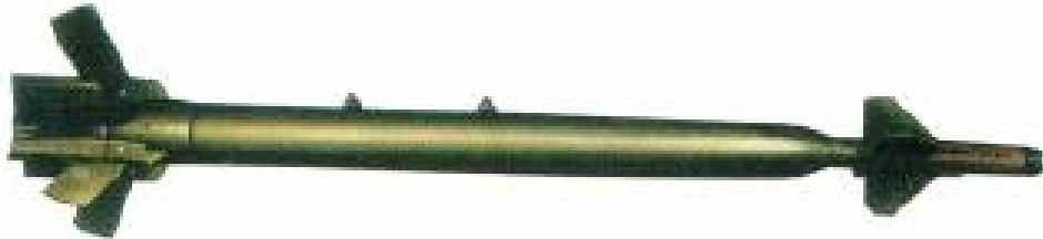
Figure 12: GBU-28 employing explosive filled BLU-113 warhead with fineness ratio of 10.5
