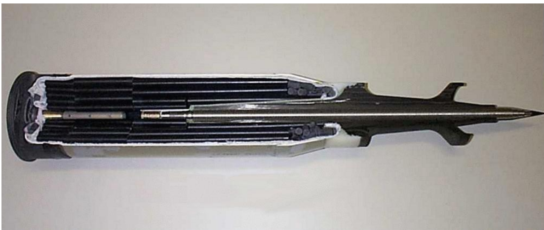
Figure 13: Anti-tank long-rod penetrator in 120 mm sabot/shell system (M829A2 APFSDS-T) with fineness ratio of about 30
