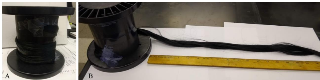
Figure E1. Photographs of stabilized bi-component fiber tow via joule heating; (A) and (B) 6000 filaments.
