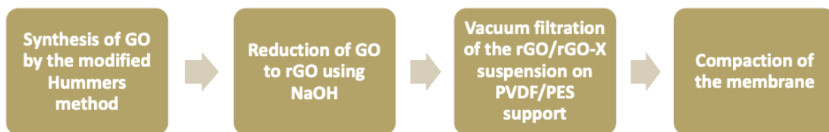
Figure 3.1: Steps involved in the fabrication of the membranes.
