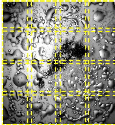
Figure 14 Stage translation in the X or Y direction between one field of view to another generates an overlap of 10%.
