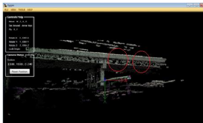
Figure 1.2: Poor quality of a generated point cloud: existence of holes
