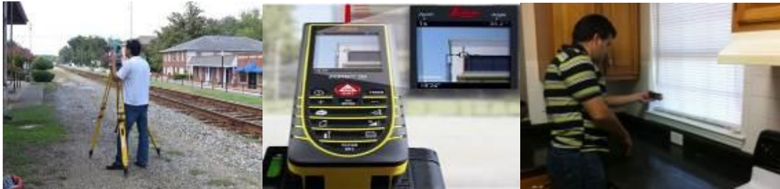
Figure 5.2: Actual distance measurements and preparation of ground truth: Leica TC805 total station (left) and Leica DISTO D5 Laser measurer (middle and right)
