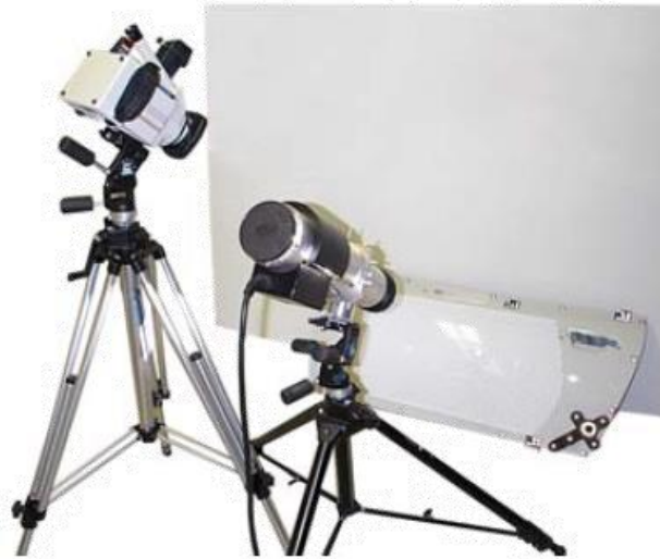
Figure 2.7: Projector and camera setup for extracting absolute measurements in manufacturing industry (Ganci and Brown, 2008)
