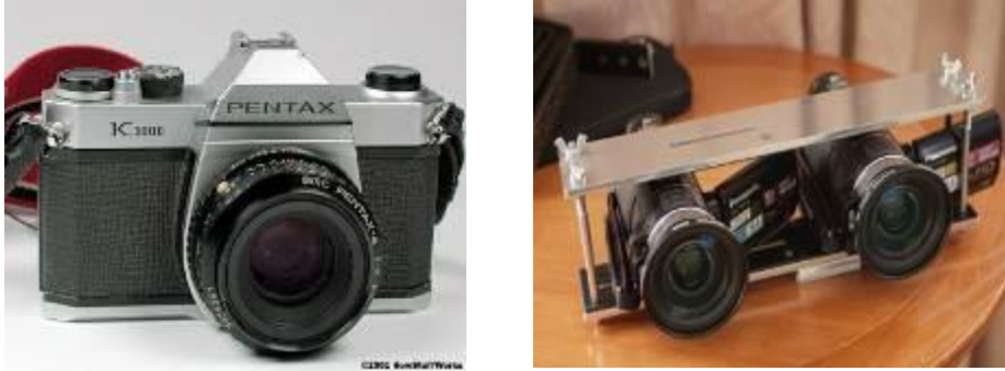
Figure 1.1: Different types of 3D reconstruction methods based on the number of applied sensors: monocular (left) and binocular (right)
