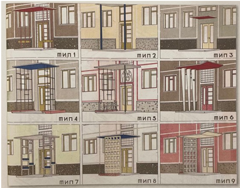
Figure 6: Nine entrance variants for the I-335, demonstrating range of color and material for exterior modular elements. Source: Meuser and Zadorin 2016.
