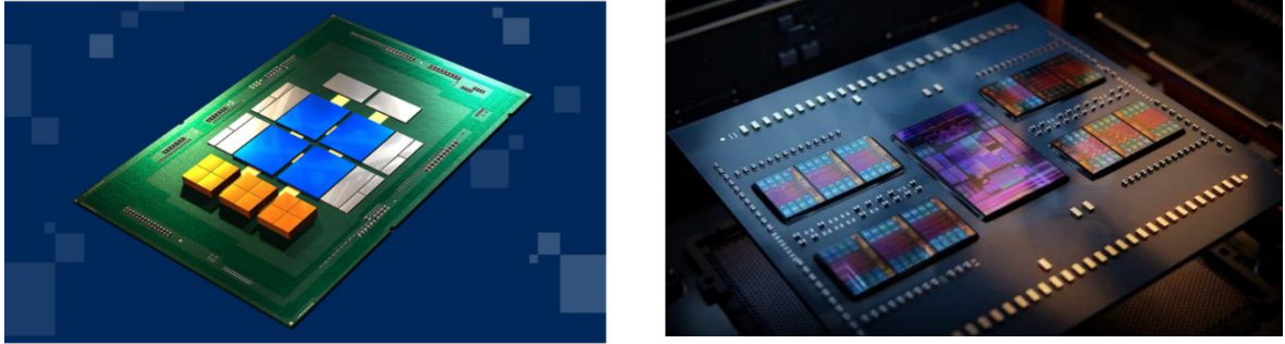
Figure 1a and 1b: Intel and AMD Chiplet Schematics (AMD offer 96 5.0 nm Cores across 12 chiplets).
