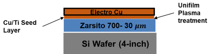
Figure 17: Peel Test Sample Schematic.
