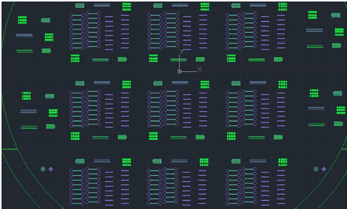
Figure 14: AutoCAD schematic of M2 (in purple) on top of M1 wiring layer in the Tri-layer stack-up.
