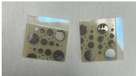
Figure 7: ITO Glass slide samples after Leakage Current and HAST measurements.
