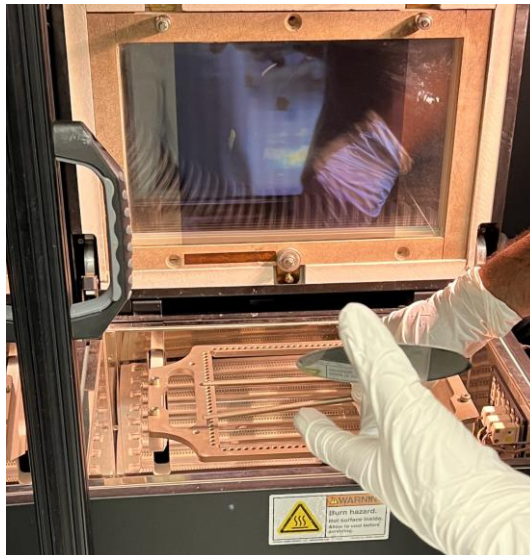
Figure 33: Akrometrix shadow moire setup in PRC with the inner sample holder/grating setup shown.
