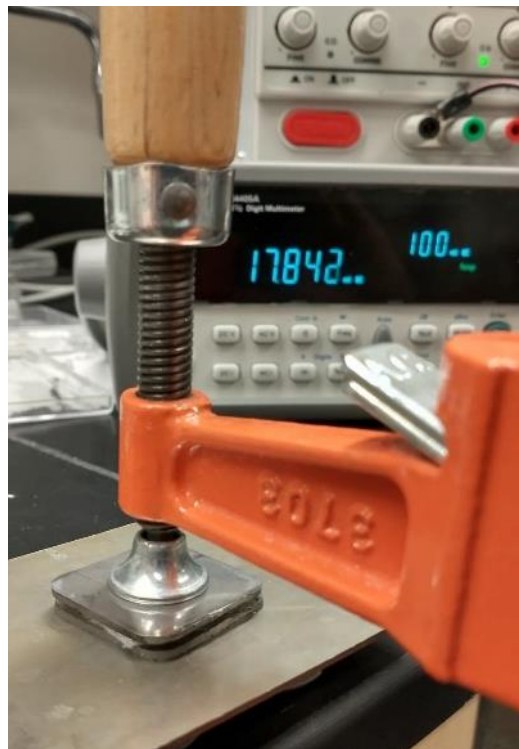
Figure 4.1 Screw press (foreground) used to exert a one-dimensional pressure gradient in dewatering experiments. A force sensor (readout in background) allows precise control of the applied stress.
