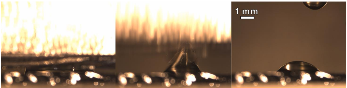
Figure 3.9 Dynamic transfer can be used to transfer liquids against the wetting gradient. By separating the surfaces quickly, 30% of a droplet initially on a silicon oxide surface can be transferred to a fluorocarbon deposited surface.
