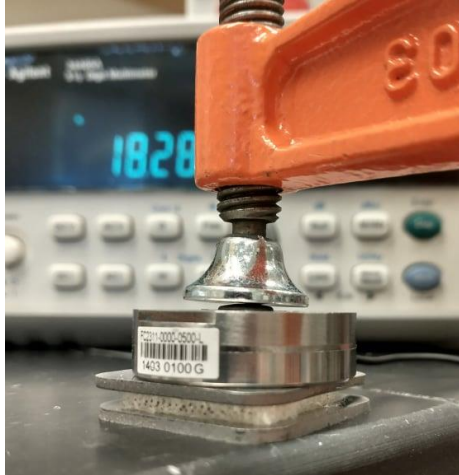
Figure 5.1 Screw press used for dewatering trials. From bottom to top are seen: the bottom platen, paper, press felt, top platen, force sensor, and screw press.
