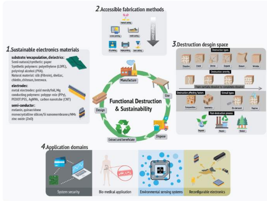
Figure 6.2: Overview of the design space for functional destruction, including detailed destruction types, sustainable electronic materials selections, available fabrication methods, and the potential application spaces.
