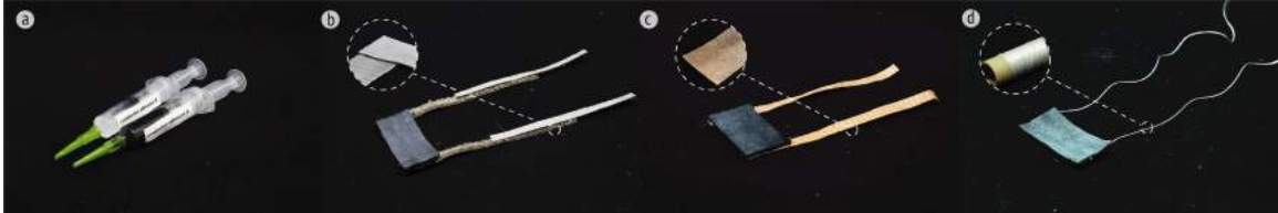
Figure 5.5: (a) Two parts of the instant conductive adhesive; (b) Conductive hook & loop connection method; (c) Conductive fabrics connection method; (d) Conductive thread connection method.
