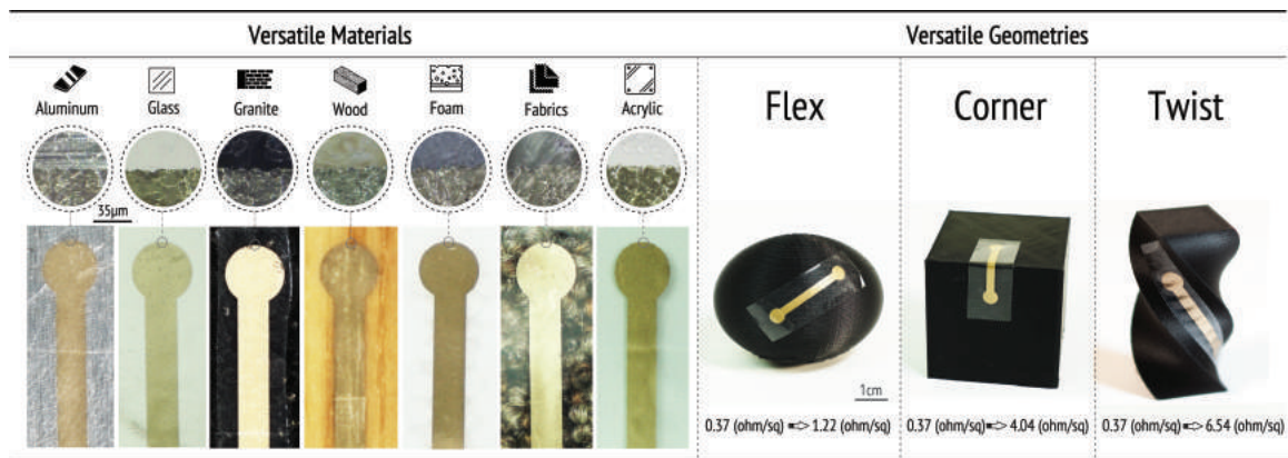
Figure 3.5: Silver traces transferred onto different materials and geometries.
