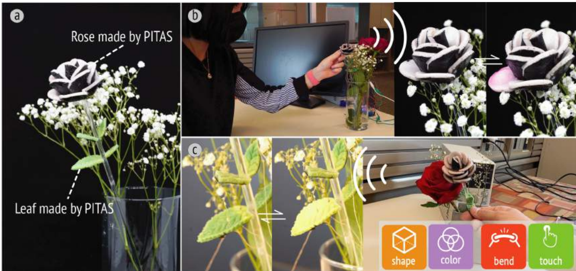
Figure 5.11: (a) Overview of the artificial rose and leaves fabricated by PITAS; (b) Delivering color change (colorless to pink) and flower blossom to partners remotely when missing each other; (c) Delivering the depression by enabling the color change (green to yellow) and leaf hanging down remotely.
