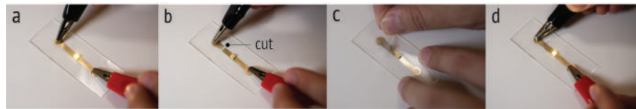
Figure 3.4: (a) Silver trace is transferred onto PDMS and connected with LED. (b) Part of the trace is removed. (c) Recovering the damaged portion with a new silver trace. (d) The silver trace is recovered.
