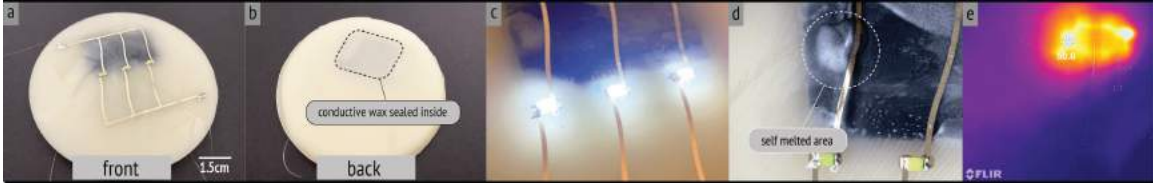
Figure 6.9: Demonstration of creating a self-destructing circuit from Beeswax: (a) The front LED circuitry side; (b) backside to show the Beeswax-graphite composite is sealed inside; (c) The LEDs are on; (d) The circuits are damaged and the LEDs turn off. (e) The Beeswax-graphite heater reaches 50°C under thermal camera.
