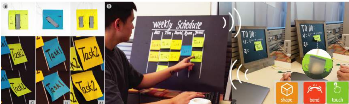
Figure 5.12: (a) Different actuation modalities; (b) Remotely synchronize the task progress by tapping or bending the Post-in note with PITAS attached on the back.
