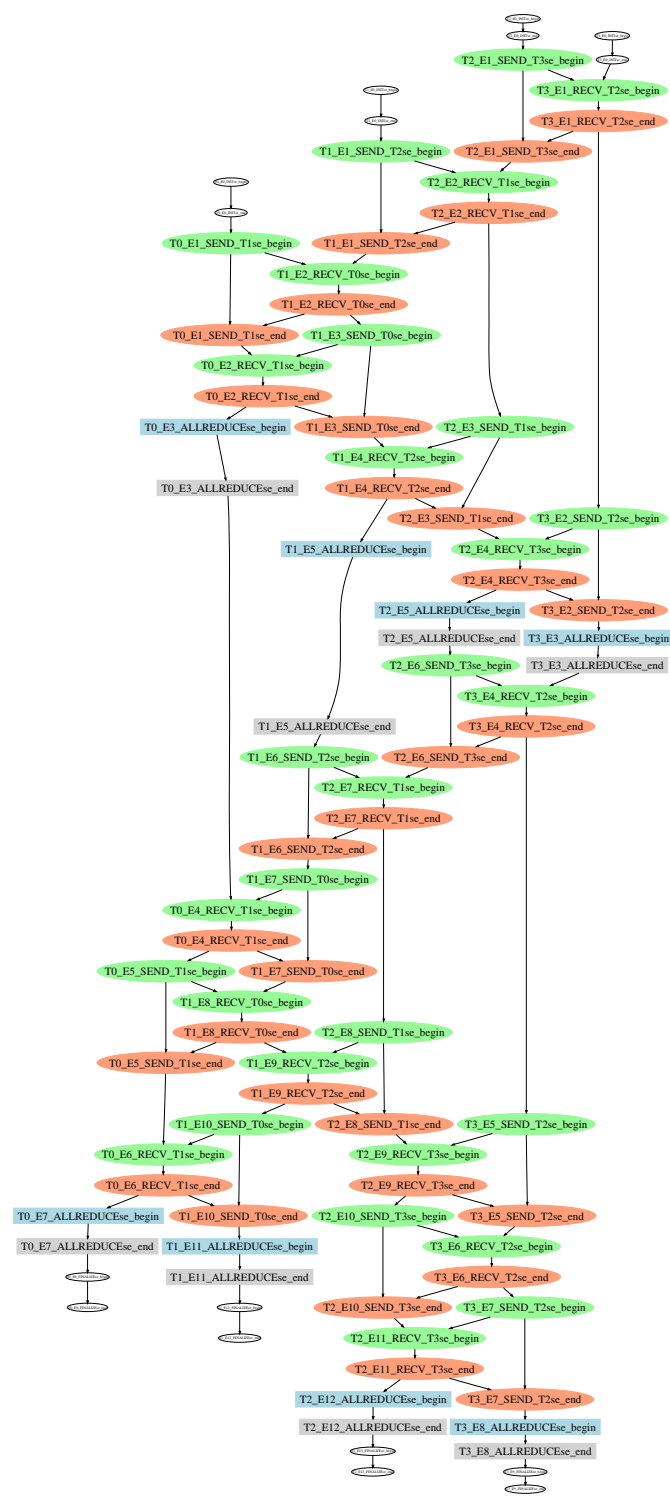
Figure 5: A Message-Passing graph for Trace Data containing Blocking MPI Primitives.
