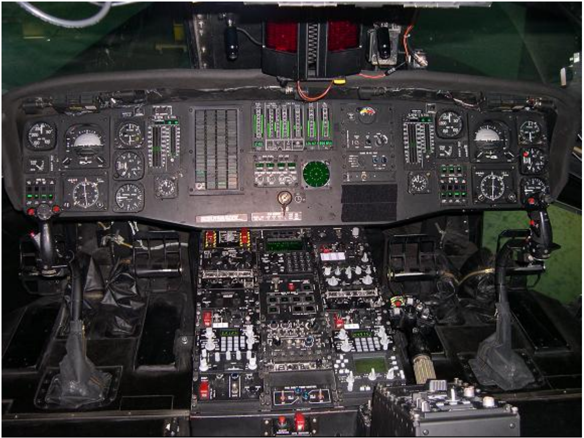
Figure 5.1: Cockpit of the NUH-60 Black Hawk Simulator
