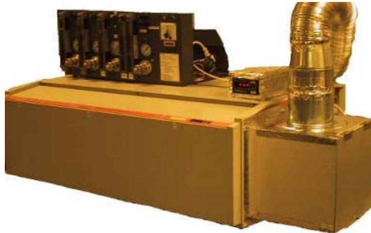
Figure 26: Mini brute annealing furnace from Thermco Inc. with a customized fume hood and a flow meter system.
