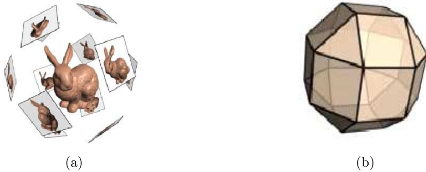
Figure 3: Illustrations of the calculation of SSE: (a) An example of 12 camera views surrounding a 3D object, where the viewpoints and view orientations are uniformly distributed; (b) The 24 vertices of the small rhombicuboctahedron are used as the viewpoints in the evaluation of SSE. These pictures are courtesy of Linstrom [63].
