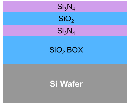
Figure 22 – Material stack used for device fabrication: a silicon substrate with a wet thermally grown SiO 2 layer, followed by two LPCVD Si 3 N 4 layers separated by an ALD-deposited SiO 2 layer.
