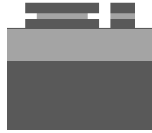
(8) Remove PMMA to reveal final device structure.
