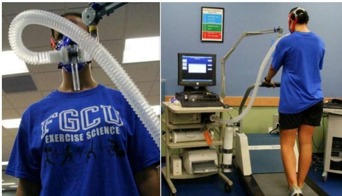
Figure 1 - The PARVO system with required facemask (Left) and the associated cart (Right) responsible for processing the exhaled gasses
