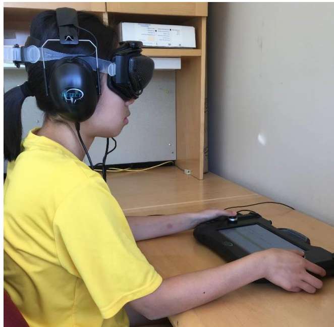
Figure 2. The Display Enhanced Testing for Cognitive Impairment and TBI (DETECT) is a neurophysiological assessment tool with 8 subtests. It is comprised of a headset, headphones and a controller with two main buttons for answering prompts.
