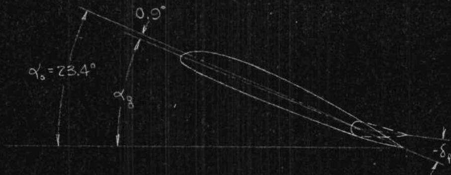
FIG. 1. b. BLADE SECTION AT \frac{3}{4} RADIUS (M-G AIRFOIL SECTION) SHOWING 20% PLAIN FLAP.
