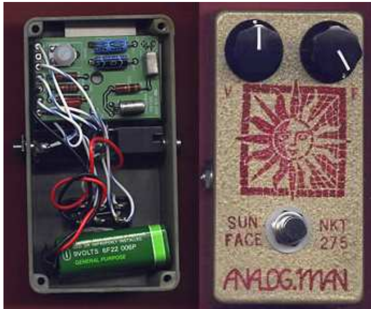
Figure 2.1 – A modern example of the Fuzz Face circuit and its housing [5][6]. Photo used with permission.
