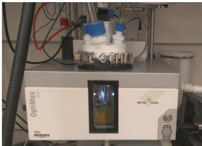
Figure 7.2: 250 mL reactive crystallization set up.
