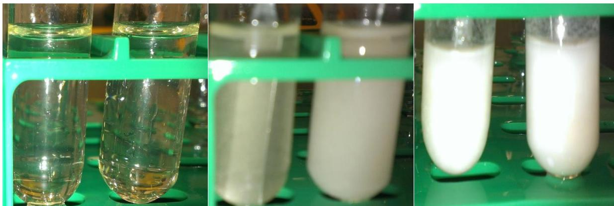
Figure 7.17: Picture of reactive-crystallization Run 4 and 5 when reaction started (left), after seeding (center), and after 6 hours (right).
