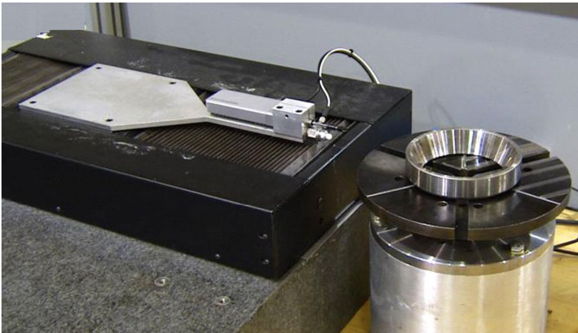
Figure 3.1 - Prototype System: Spindle, Linear Slide, Measurement Probe, Pusher Tip
