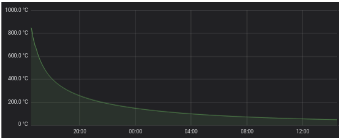
Figure 26: Transient cooling from 850°C after a completed print
