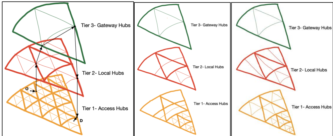
Figure 2: Flow of goods in a hyperconnected network for city logistics with radial pixelization under (a) uniform demand distribution, (b), (c) radial demand distribution varying inversely with square of radius.
