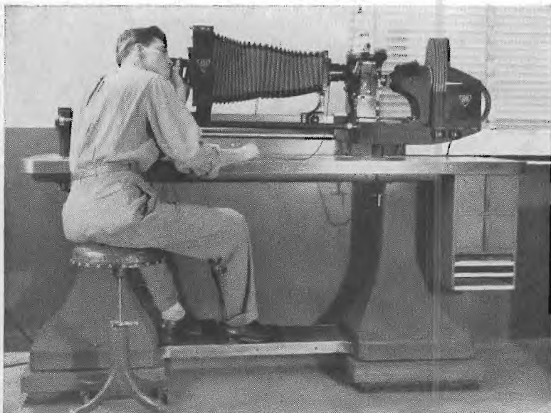
Co-operative student examining metallographic samples, Research Laboratory, International Nickel Company, Huntington, West Virginia.
