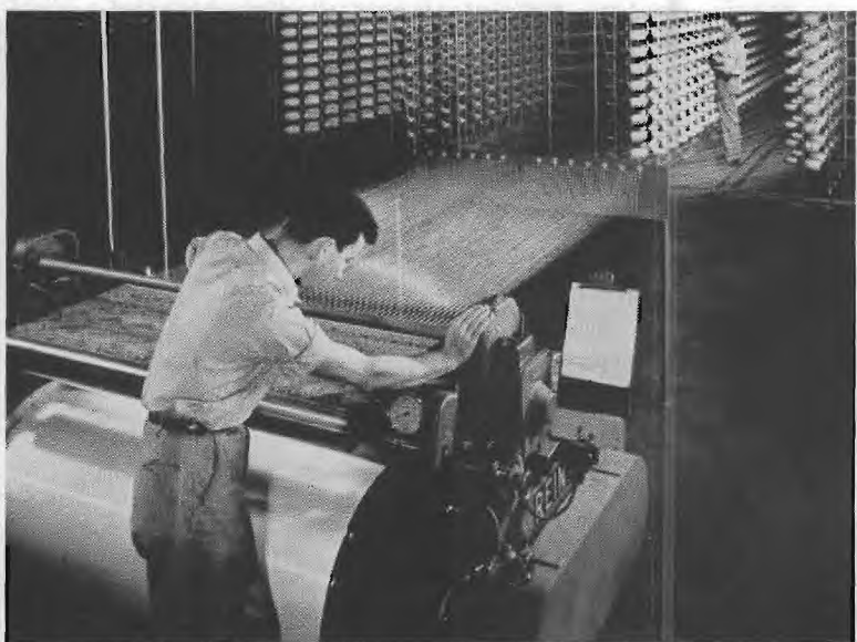
Section Beamer and Creels in yarn plant of Tennessee Eastman Corp., Kingsport, Tenn., where Co-operative students get training.
