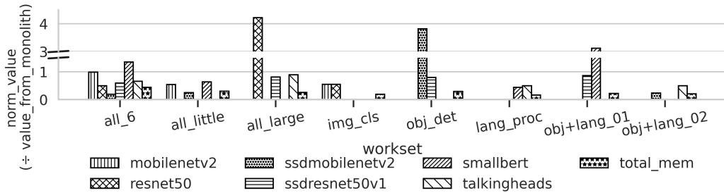
Figure 3.9: To evaluate how Pocket works when serving multiple applications, we create 8 workload mixes. Each one of them is a subset of the 6 models that we use in the earlier experiments. The y axis shows the normalized value of Pocket compared to a monolithic Docker deployment for application latency and total memory usage (total_mem). Lower is better. Overall, Pocket leads to shorter latency results and shows reduced memory usage, compared to the monolithic approach.
