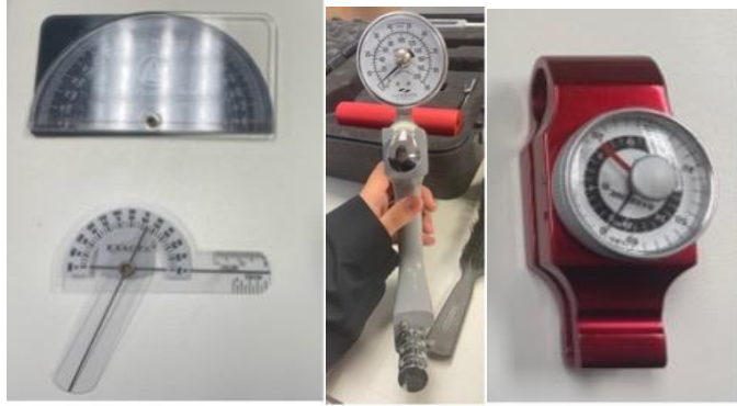
Figure 1 - Goniometer, dynamometer, and pinch gauge tools for hand measurements.
