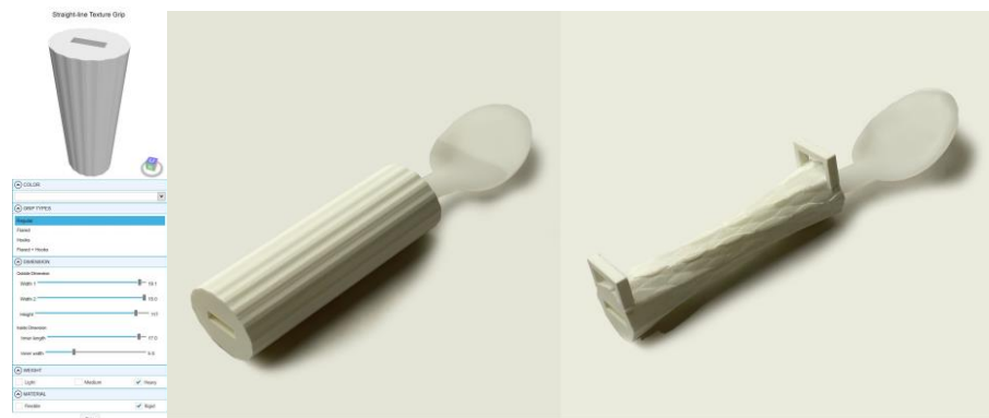
Figure 7 - The left image displays the outcome of the interface's manipulation of a grip by the OT, while the right image exhibits the printed grips attached to utensils.
