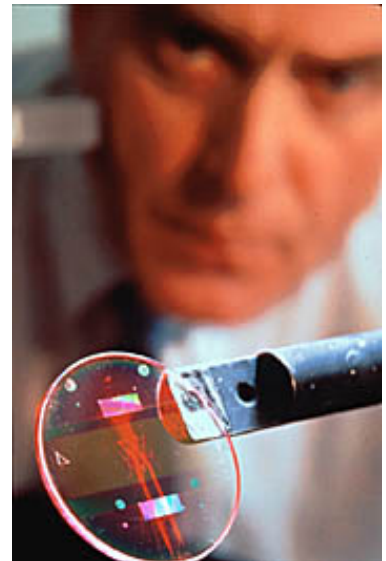
An integrated optic interferometric sensor, developed by GTRI scientist Nile Hartman, quickly detects even the smallest amounts of various contaminants in air, soil, groundwater and food. ( 300-dpi JPEG version - 323k )
