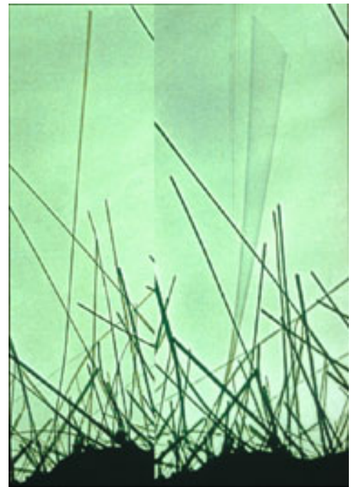
A transmission electron microscope image shows "nanobalance": a resonating carbon nanotube used to determine the mass of the attached carbon molecule.
