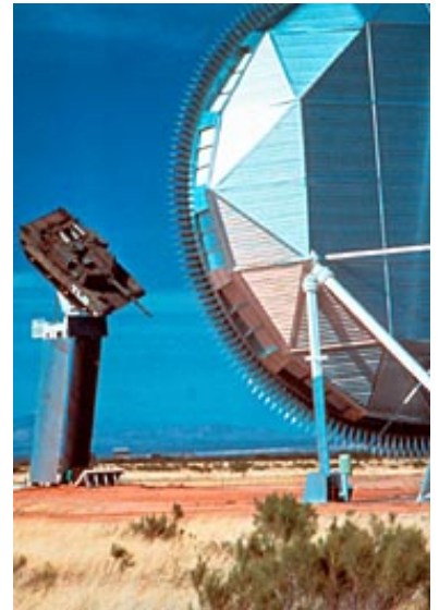
At Fort Huachuca, Ariz., the U.S. Army constructed a compact radar range thought to be the world's largest. GTRI scientist Dr. R.C. Johnson invented the compact range in the late 1960s.
