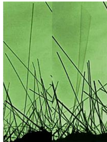
The images above show a bundle of carbon nanotubes (left), and the same bundle to which an oscillating current has been applied (right), causing resonance in one tube.
