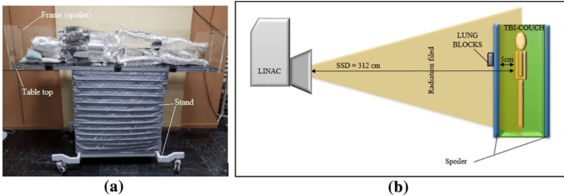
Figure 2. Total body irradiation (TBI) setup for Linac-based AP/PA geometry: (a) lateral view of the phantom on a specifically constructed TBI couch including tabletop, stands, and therapeutic frame, in the treatment room; (b) position of linear accelerator (LINAC), phantom, lung blocks, TBI couch, and radiation field. 7
