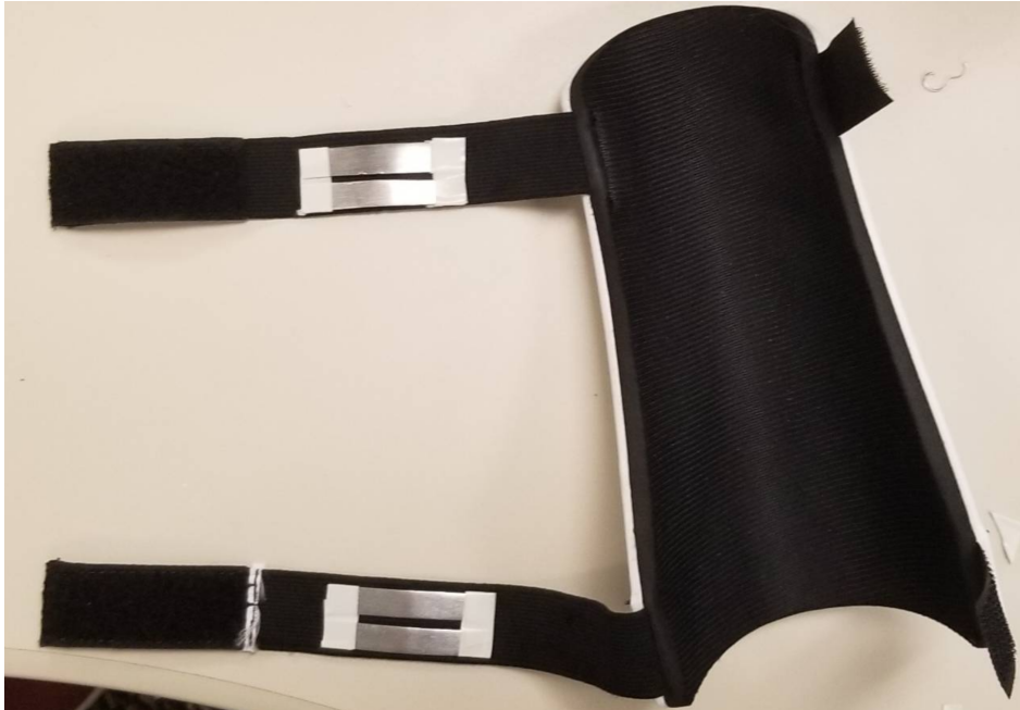
Figura 1: Smart Shinguard with two sets of dry electrode placed on the straps to attach to the back of the calf
