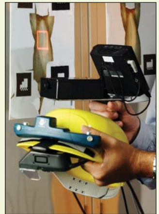
ABOVE: One augmented reality system developed at Georgia Tech uses a location-tracked, see-through, head-mounted display (foreground) worn by poultry workers. It directly overlays graphical instructions on a trimmer's view of the birds.
