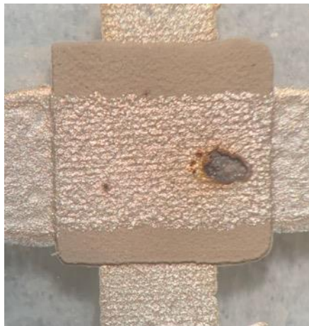
Figure 8 Dielectric breakdown in poling process: Microscopic surface image of affected device.
