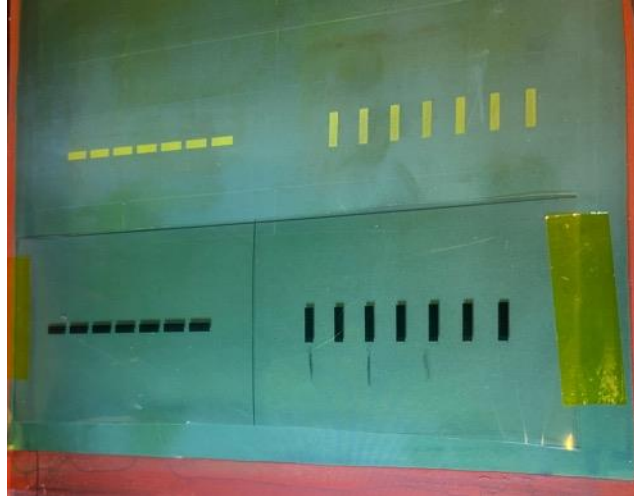
Figure 4 Transparent patterning masks and 200 mesh count screens: Key elements of the screen printing process.
