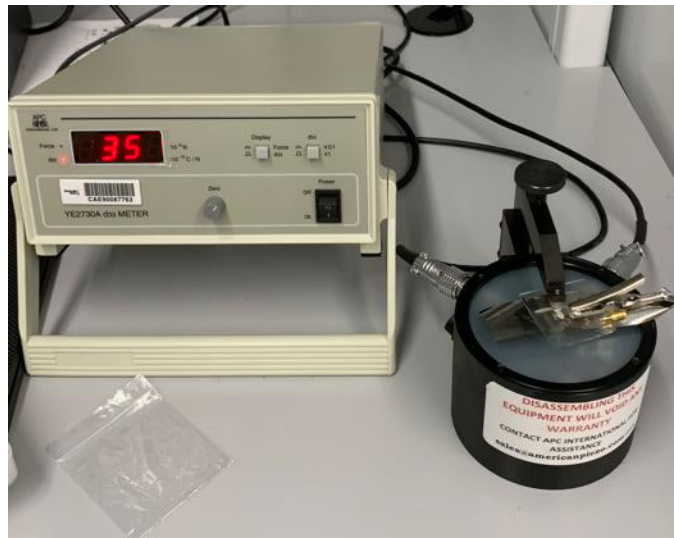
Figure 23 Piezoelectric charge constant measurement setup with d_{33} meter.
