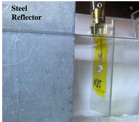
Figure 29 Measurement setup for pulse-echo measurement with steel reflector.
