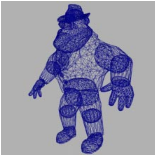
5 d. Wireframe of Original Model (shows intersecting parts) 13,476 Faces
