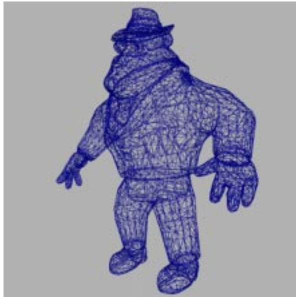
5 e. Wireframe of Repaired Model (shows manifold surface) 13,476 Faces
