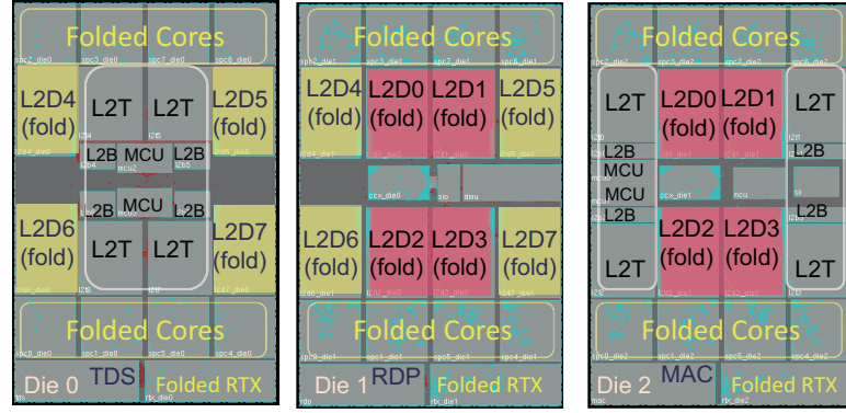
(a) 3-tier folded modules (Core and RTX) and L2$ floorplan
