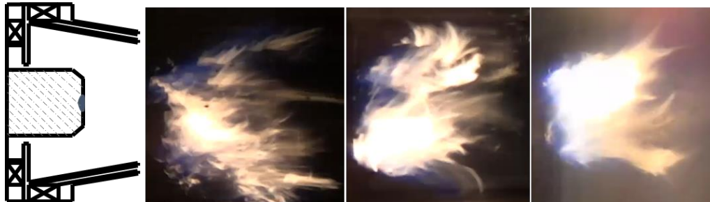
Figure 5.1: Instantaneous camcorder images of the A-2 flame at the 300 K (left), 450 K (center), and 550 K (right) air inlet temperatures.
