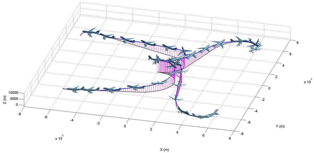
**Figure 12:** 3D glider landing trajectories generated in DENMRA.
