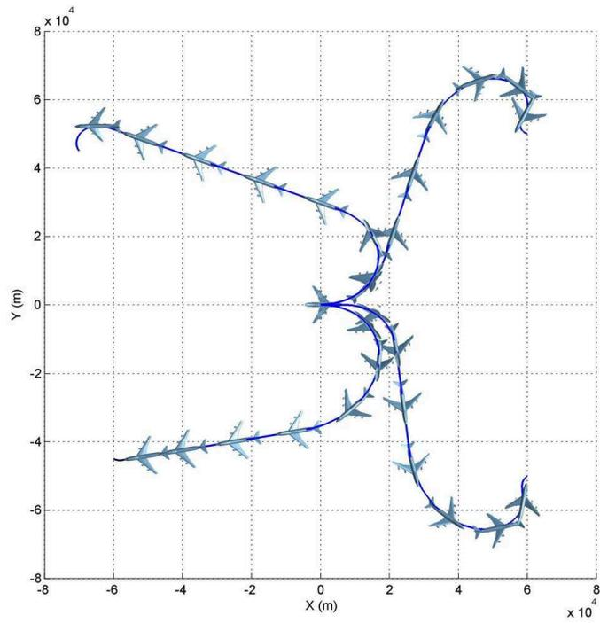
**Figure 13:** 2D projection of glider landing trajectories generated in DENMRA.
